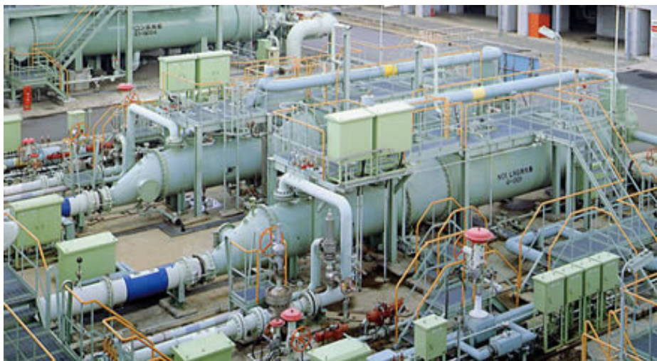
Figure 8: Typical self-contained IFV installation using seawater for heat source (See Fig 7 for schematic diagram)
