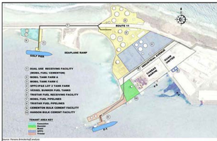
Figure 16-6. Fuel Receiving Infrastructure at the Port of Guam
